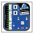
Once the pump has been powered on, simply use the up and down buttons to select the desired Lubrication Cycle. There are 12 different cycle times that can be selected:
